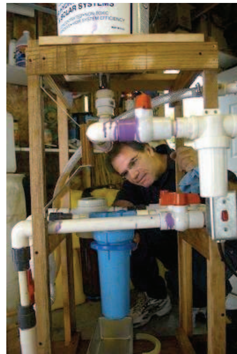
Jim Gill checks out a homemade device used to filter vegetable oil he burns in his modified Jetta. Photo/ Keith Hale/Sun-Times
